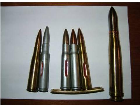
very similar at first glance – which might be confusing for those who are not cartridge collectors. (The easily recognisable difference is the belted base of the Boys round. Belted cartridge cases are rare in military weapons and are used where immense strength is required in order to withstand high internal pressures when firing.)
