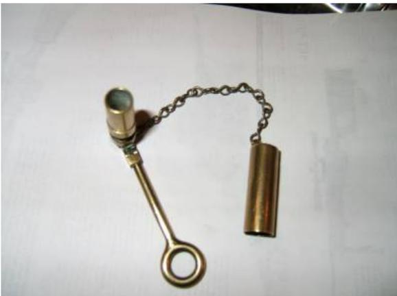
Mike also provided a “Sergeant’s Tool” – a brass tool with a swivel mirror attached at the one end for inspecting rifle barrels. It dates from the pre-WW2 era.
